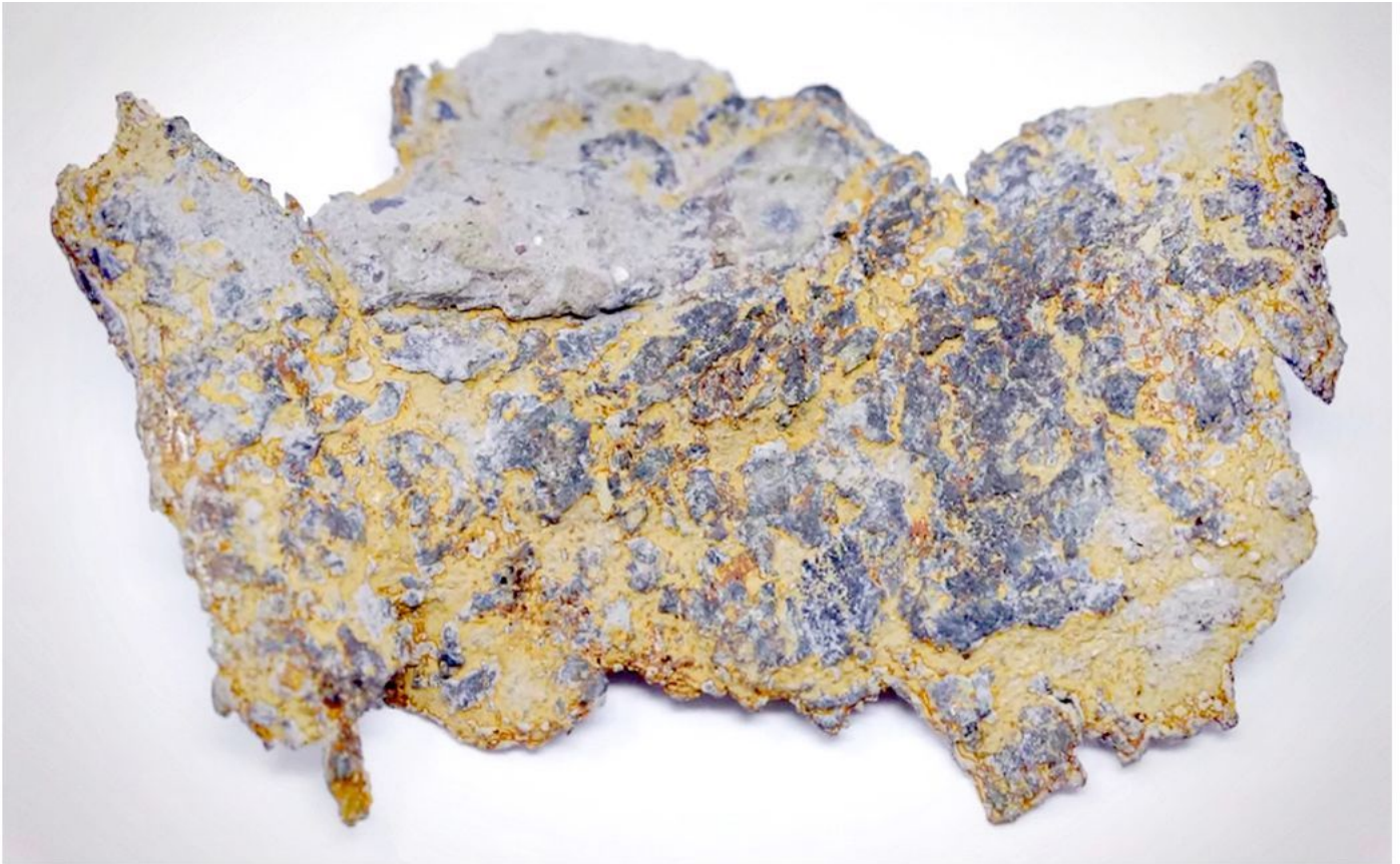
Geopolymer limestone Cladding on iron Borehole D2
