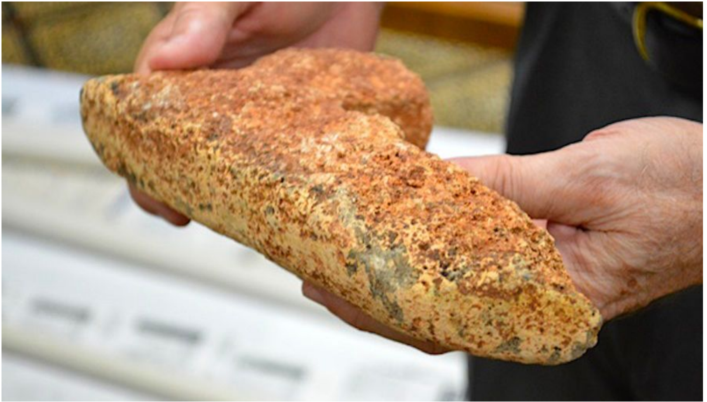
Pavement tile, ferrite-coating Geopolymer limestone Edmond, Oklahoma
