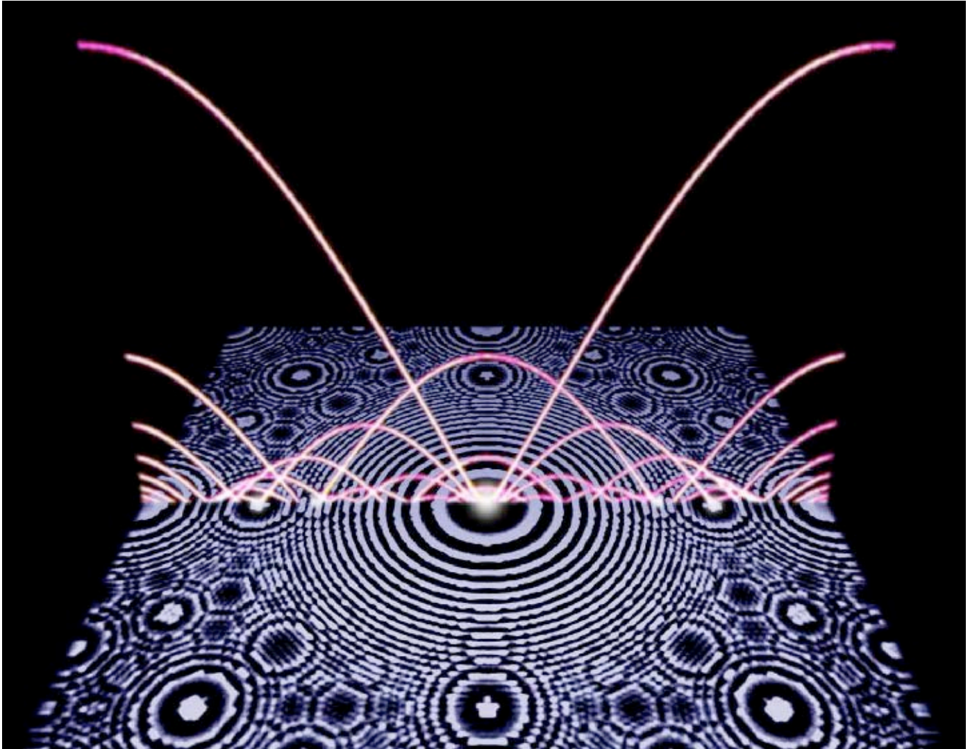
Cross-section of nonlinear standing waves (in pink) and their acoustic pressure distribution pattern (in blue)
