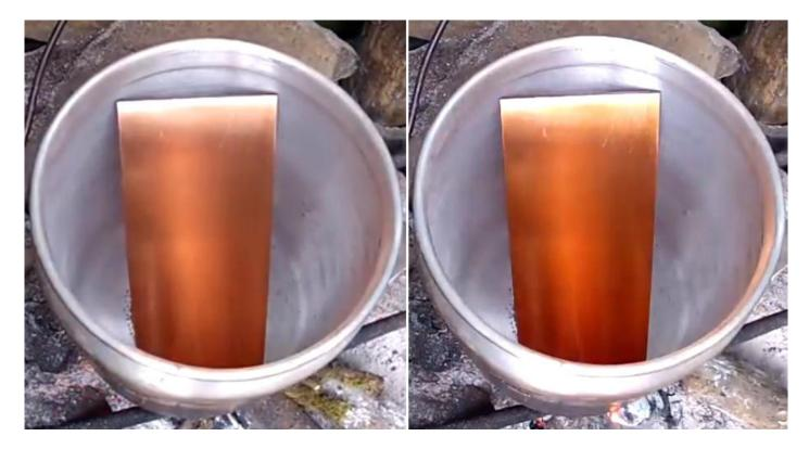
Ultrafine gold nanocoatings achieved by artisans of the Nariño and other Andean cultures were made by keeping the metalworks under visual observation during heating in ceramic pots on a wood fire, and quickly removing them from the pot with tongs immediately after the appearance of orange gold formation. This was then repeated a second time after a cooling period of just a few minutes.
